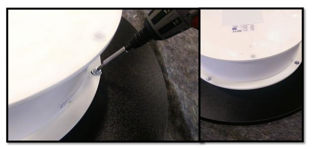
**Step 3: Turn the screws into the presentation disc**Please make sure that you cover each hole with a ring before you start screwing.
